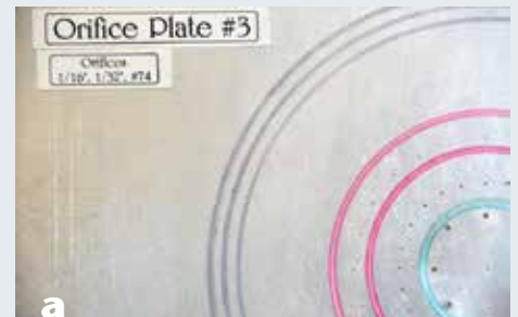
This orifice plate has eight \frac{1}{16} " holes within the inner green ring, 24 \frac{1}{32} " holes between the green and red ring, and 24 No. 74 holes barely visible between the two red rings. The smallest holes allow measurements at lower leakage rates. The holes should be spaced about \frac{1}{4} " apart to prevent airflow interference between them.
