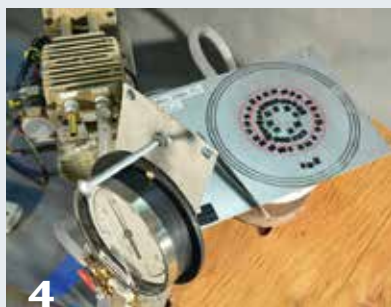
To assess a pump's airflow, use large tubing to connect it to the vacuum chuck. Fit the vacuum gauge in a separate port on the side of the chuck. With the pump running, uncover the desired number of orifices of the same diameter and record the vacuum level. Run repeated tests, each time uncovering the same number of same-sized orifices and covering the previous set. This photo shows three \frac{1}{32} " orifices opened.
