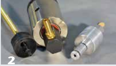
A rotary vacuum adaptor ties the rest of the system into the lathe. Three manufacturers make these adaptors for the same lathe. Notice the differing methods implemented to achieve similar functionality. The adaptors are oriented to show the critical orifice, or narrowest opening, for each. The unit on the left will have an airflow estimated at about 30% of the unit on the right.
