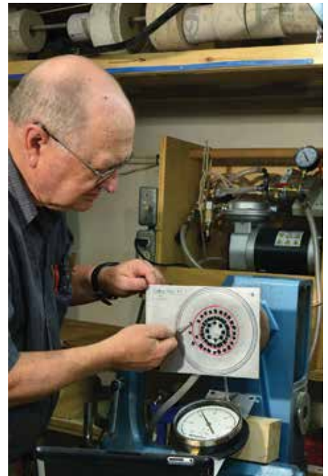
The author uses an orifice plate mounted on a vacuum chuck to measure the airflow rate into the system. This test entails systematically opening orifices on the plate, taking readings on a vacuum gauge, calculating airflow, and graphing the data.
