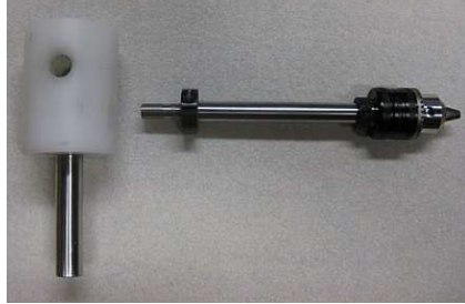
Two stop collars, drill chuck, and cold rolled steel rod threaded at end.
