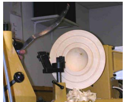
The Kelton Bowl Saver system in place. The base is in the toolrest and lined up with the inner-most cut. The tool (shown over the bowl) has been ground with a diamond-shaped bit.
