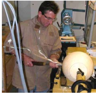
Turning the outside of the wet blank using a 3/4" gouge with a fingernail bevel. Notice the shavings flying off.
