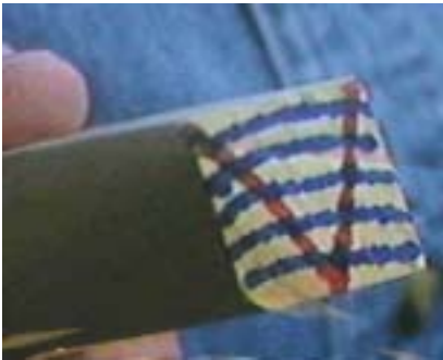
Showing how the grain will align with each piece, and the "V" showing how the piece will be chamfered. John uses 60° chamfer bits in his router table, being careful to clamp feather boards and support boards to support the sides and top of the long narrow stock as it is fed through the router. However, he says you can get a 4-part laminate just using good birch quarter-round molding without requiring any premachining of the stock.
