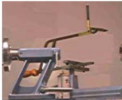
Don's hollowing setup, with adjustable laser guide and solid tool rest. ❖
