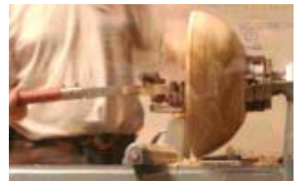
Carefully aligning the tool in the McNaughton jig, Allen starts to core out the blanks, starting from the center. He uses the tool that most closely matches the inside curve of the piece being removed. After removing the blanks, Allen stacks them face down on a concrete floor until they dry.
