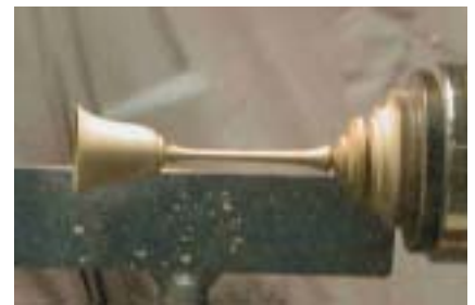
Side view of goblet. All shaping and sanding for the bowl must be finished before the stem is turned.
