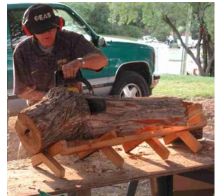
Picture of Jerry's bucking stand. He prefers to work at waist height if possible and sized his stand to place it on a table if desired. His stand is a series of crossed supports with side beams to hold them together.
