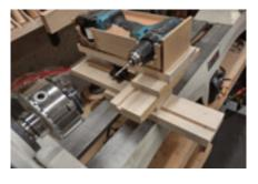
locks in place) and the drilling action. He molded a urethane pocket to hold the drill.
