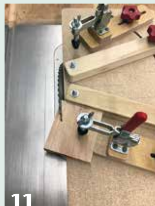
Always register the top, or wide, end of the stove against the fence—never the smaller end. Adjust the hold-down position and clamp the stove in place. Use a steady, even pressure to cut the first side.
