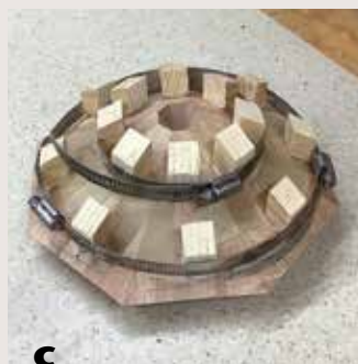
c Hose clamps draw the glue joints tight. Dry-fit the assembly first to get a feel for sufficient pressure.
