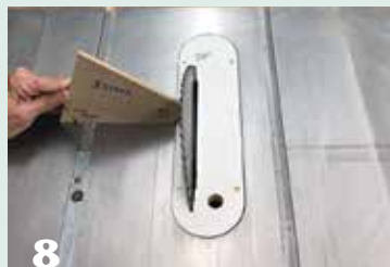
8 A single set-up wedge is used for both blade and fence angles. Set the blade angle using the small end of the set-up wedge.
