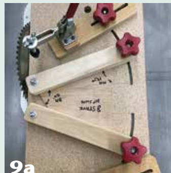
(9-9a) The long sides of the wedge are used to set first the lower fence, then the upper fence. The wedge ensures easy, accurate setup every time.
