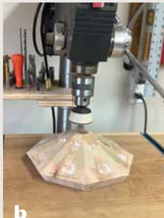
b The base can be flattened using a drill press with a sanding disk.
