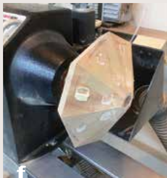
e Because the jaws will hold the workpiece in expansion mode, only a small recess is needed.
