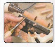
Use a gouge to rough turn the blank to a cylinder.
