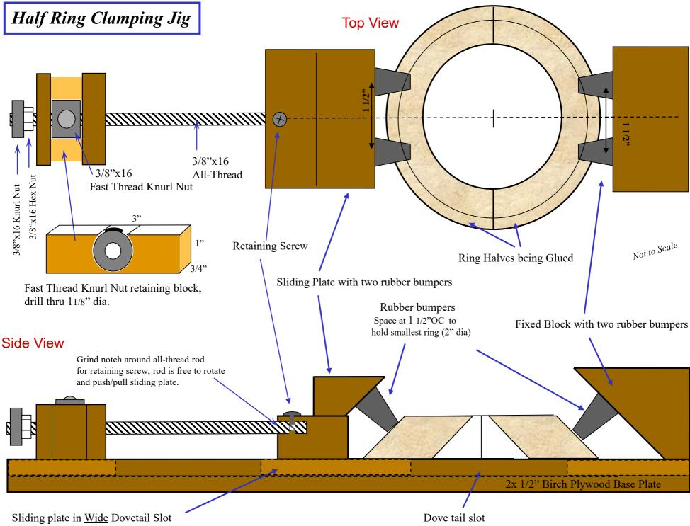
(top piece of 1/2" ply: two 45° cuts form dove tail slot)
