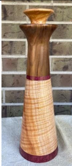
Crush Grind Peppermill - The body is Figured Maple framed with bands of Purpleheart. The neck is Walnut. This was loosely patterned after the "Classic Vinegar Bottle Peppermill" described in Chris West's book on pepper mills. I have several more in progress utilizing various combinations of wood. – Bob Britt
