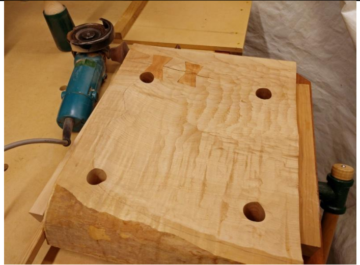
Power carving a shop stool seat from 3 inch thick maple hunk. Mahogany butterfly inlays. – Al Murphy
