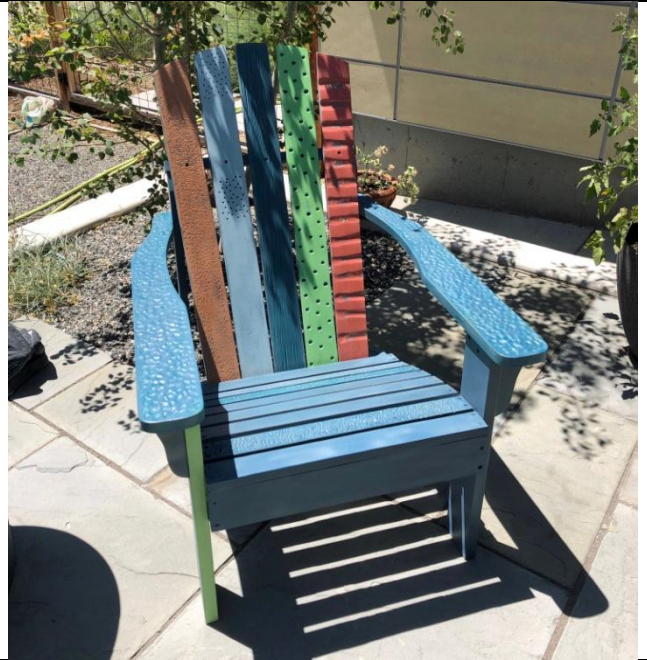
Decorated chair for old town Louisville. Used a full repertoire to texture: countersink for polka dots, drill bit for holes, v tool to make lines, Rotary grinder to do arms & seat slats, engraver for wiggly lines. Finish: milk paint mixed with acrylics to tint, General exterior satin finish. – Merryl Saylan
