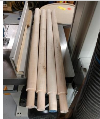
Also working on a 4-legged stool, rough legs made from wormy soft maple. Al Murphy
