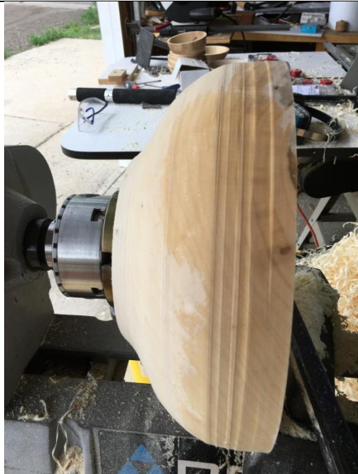
Attached are more pictures of the ongoing processing of wet silver maple into rough bowls. I may be taxing my Delta 1440 as there are a lot of grumbly noises coming out of it. If anyone knows how to work on these lathes I'd really like to talk to you. 775-741-0418 – Jason Matisheck
