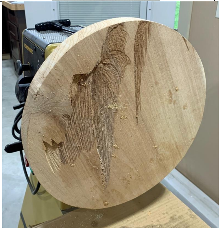
Here is a platter I made out of a blank someone gave me. The blank started out at about 1\frac{3}{4} " but was really a ragged cut (See right) had a pretty deep screw hole on the other side.. By the time I got the ragged cuts out of it, and got the screw hole out, it was down to less than \frac{1}{4} " on the bottom. It is not quite smooth on the inside, but I was afraid to cut anymore off of it! – Robyn Herman
