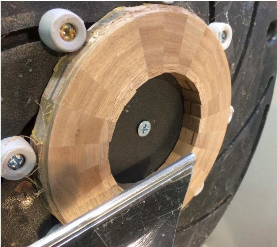
Seventh photo shows row number 2 turned and sanded flat in a Longworth chuck.
