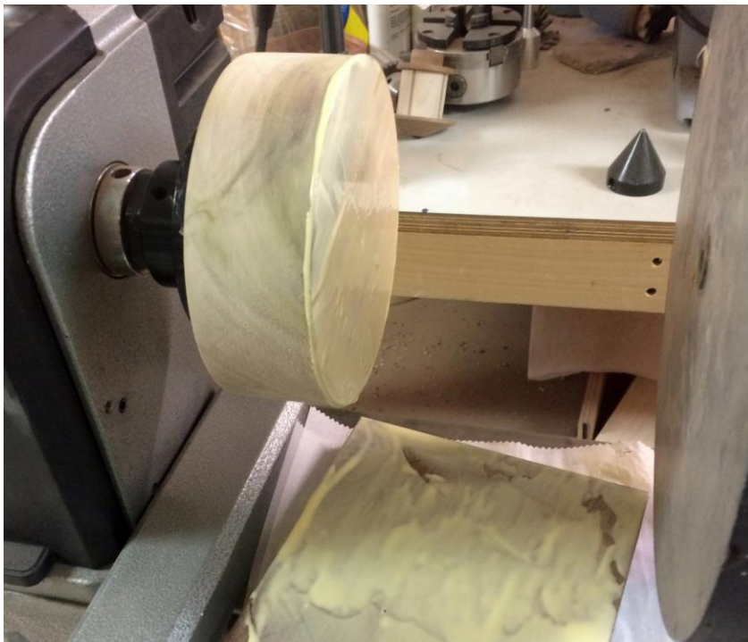
Fifth photo shows the glue block on the chuck. Glue block is turned round and sanded. The face has to be absolutely dead flat. The base piece is walnut covered with glue ready to be set. In the tail stock you see a plate. I use that to press the rings flat.
