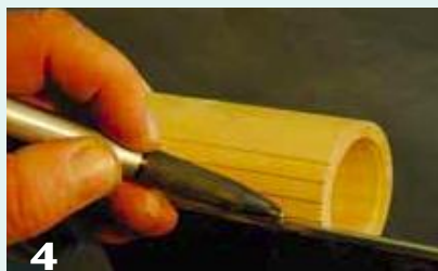
4 With the lathe's index pin engaged, draw the lines for the segments. Use a soft-lead pencil and run it along the toolrest.
