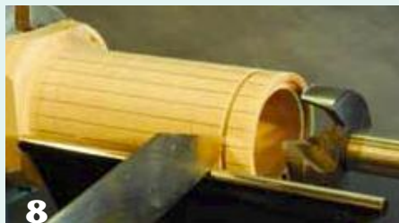
8 Using a thin parting tool, part off the first ring at the previously marked point. You should end up with a ring that is about ⅜" (10mm) wide.
