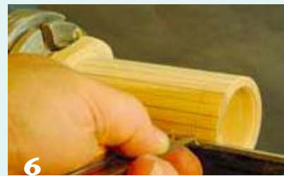
6 Starting from the tailstock end and using dividers, make a mark every ½". You should be able to mark off six or more rings.
