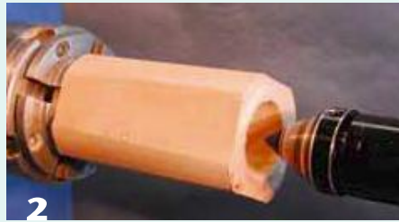
2 Use a cone center to help minimize flexing and vibration and to help compensate for any offset errors created in the drilling process.
