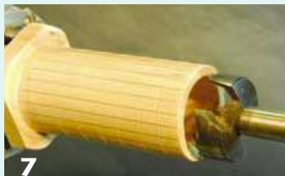
7 With a 1¾" (45mm) Forstner bit mounted in a Jacobs chuck, drill ⅝" (3mm) deep into the end of the tube to form a rabbet.
