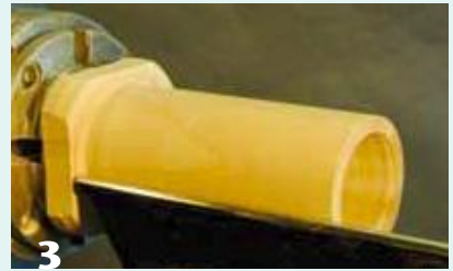
3 The wood is drilled, turned, and sanded and is ready for laying out the segments.
