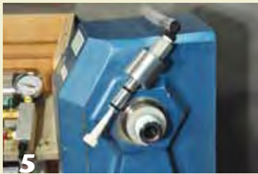
5 To test for bearing leakage through the vacuum coupling, a plastic plug can be inserted into it.
