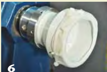
6 The chuck to bowl seal is achieved here by utilizing sheet craft foam.
