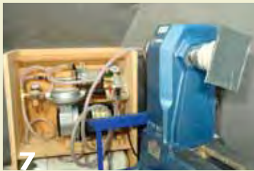
7 To test the overall system for leakage, an aluminum sheet is placed over the vacuum chuck. It tests the seal on the vacuum chuck as well as all other components and connections.
